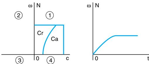
$$\begin{aligned} Ca \text{ (N}\cdot\text{m)} &= J \text{ (kg}\cdot\text{m}^2) \frac{d\omega \text{ (rad/s)}}{dt \text{ (s)}} \\ &= J \text{ (kg}\cdot\text{m}^2) \frac{2\pi N \text{ (rpm)}}{60t \text{ (s)}} \end{aligned}$$
